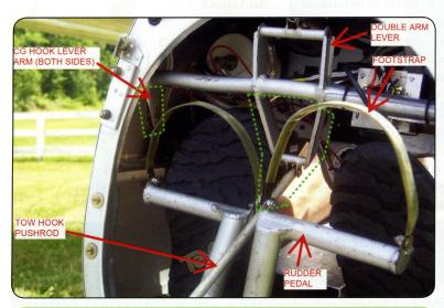
In order to avoid future inadvertent releases, it is recommended that the L13 front seat pilot use the foot straps if flying the airplane on tow. If not flying the airplane, then the feet should be positioned as to avoid possible contact with tow release.
